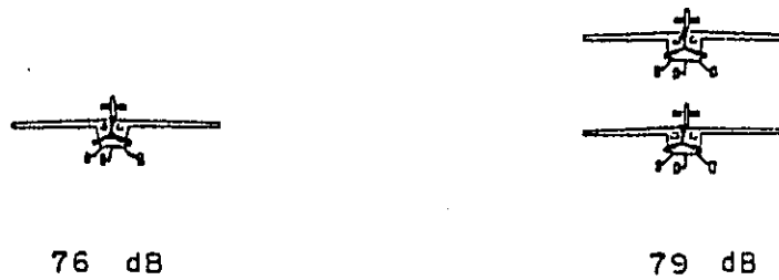
Figure 8. Doubling the number of identical sources results in a 3 dB increase in sound pressure level.
